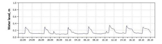
Figure xx. The example of hydropeaking in Tenenys river below Ramučiai HPP dam for period September 21 to October 20, 2020. Every few days the minimal sanitary water level is flushed by the accumulated water suddenly raising water to +20 cm. Data are taken from Lithuanian Hydrometeorological Service automatic water station in Tenenys River at Miestaliai village <u>http://www.meteo.lt/lt/hidroinformacija</u>
