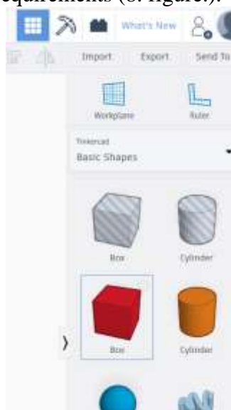
37. Figure. Choosing a standard Geometry Box using the left mouse button on your computer (once pressed on the geometry and pointing to the placement on the work plane).
